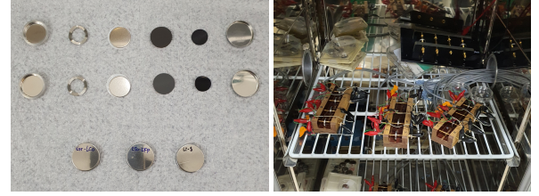
(a) Fabricated coin-cell batteries. (b) Battery testing equipment.
