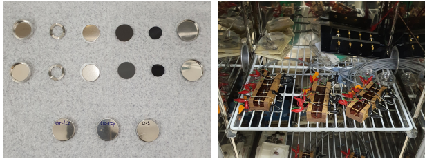
(a) Fabricated coin-cell batteries. (b) Battery testing equipment.
